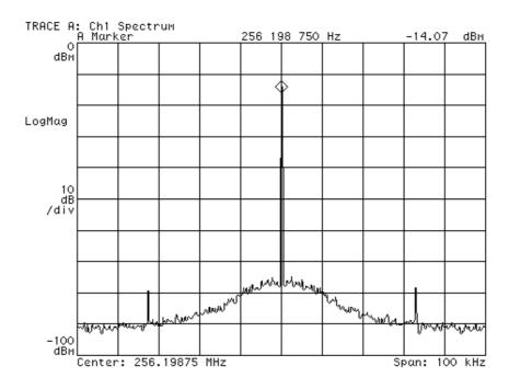
LIM\_P Measured at RIF Pin 17 (TP108) with a 10 Mohm probe:
